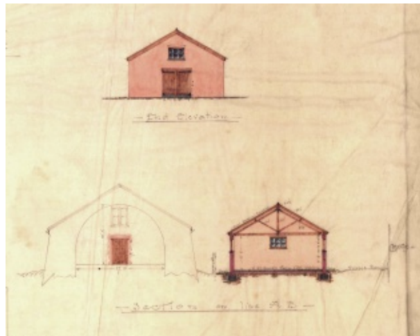
Plans for a small arms and ammunition store, 1904, in same location as existing Building B
