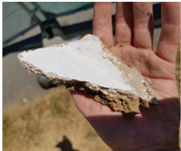
Lime outer layer of earth mortar plaster showing hair
