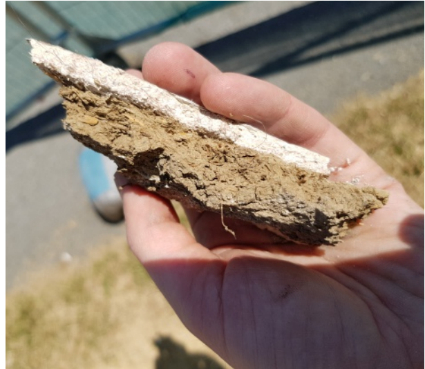
Section through fragment of earth mortar plaster
